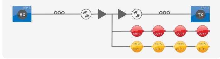
2 x Transceiver SFP with Optical convertor, each with 4 x DA output
