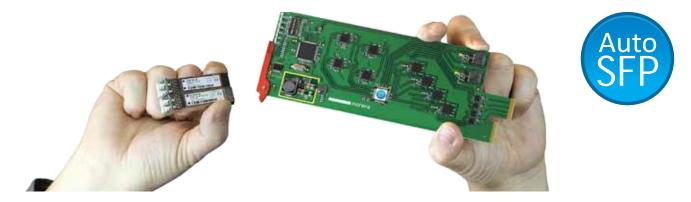
Insert a dual optical transmitter SFP, then you will have a 2 channel transmission card. Take the same Optical interface card and remove the dual optical transmitter SFP and replace this with a dual channel receiver, then Norwia's AutoSFP<sup>®</sup> technology will automatically setup the Optical interface card as a dual channel optical receiver.
