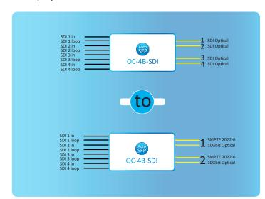
The upgrade path between SDI to optical and SDI to SMPTE 2022-6 optical is very simple with the miniHUB.
