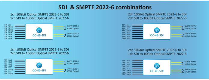
Mixed encoding and decoding solutions with the OC-4B-SDI
