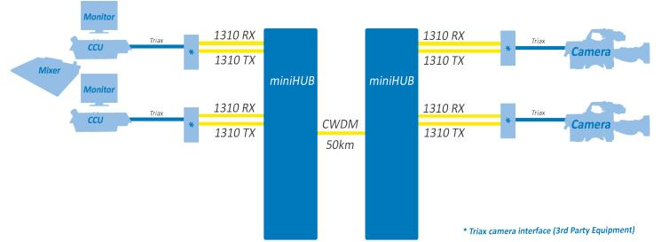
Add on Triax/Optical based systems are also good for bridging older camera systems for optical distribution networks. These type of systems can be directly mounted to the camera and eliminate the Triax part of the system.
